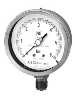
These instruments are designed for explosive atmospheres in food, processing, pharmaceutical, petrochemical industries and conventional and nuclear power plants. The MGS pressure gauges are in conformity with the essential Health and Safety Requirements laid down in European Directive 94/9/EC for Group II, Category 2G or 2GD equipment in the T1...T6 temperature classes. They are NOT suitable for ZONES 0 and 20.
